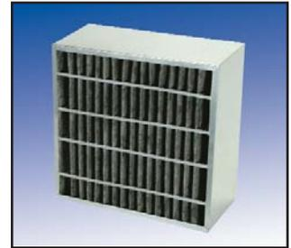
These "Rigid Cells" utilize several different types of "thin bed" activated carbon media, that are formed into pleats that are 4", 6", or 12" deep, the later being by far the most popular. The "deep" pleats are then sealed into a metal frame [rigid cell]. They can be used individually, but are normally used in a filter bank.
